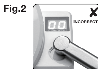
Light tip not held flat against the light sensor. Unit will display incorrect results.
